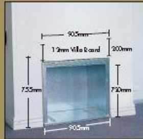
Zero Clearance Box positioned in framework mounted on 12mm Villa Board cut out size. (Box size: 905w x 720h) (Cut out size: 905w x 755h)
