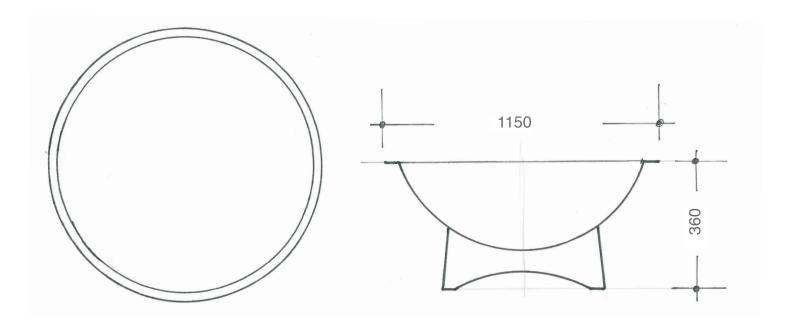
The Pati-O-Pearl bowl is manufactured from top quality P & O HA3 grade steel. It is supplied mill finish which is designed to weather over time.
